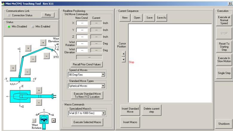
The jog section allow the User to incrementally move the arm in real time to any desired position with respect to any individual joint.
