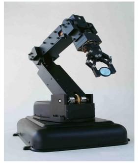
Base Robotic Arm system comes equipped with standard gripper as shown. 3D vision option is available as well as customizing end effectors, specialized application modifications and smart fixtures. Applications include pick-n-place, load/unload, pick-present object-place and assembly of light weight components, to name a few.
